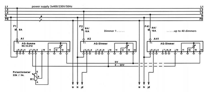
Master control with external potentiometers. The potentiometers at the dimmers can be used for the setting of individual light levels which would not be exceeded within the master function.
